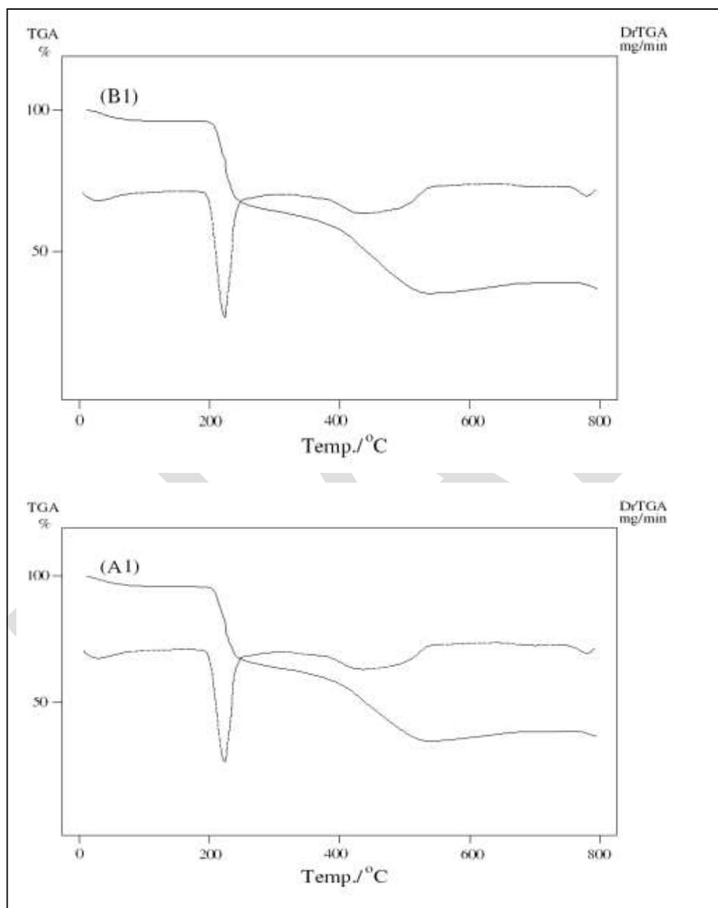
**Fig. 2: TGA/ DTG curves of copper complexes before irradiation (B<sub>1</sub>), after irradiation (A<sub>1</sub>)**
