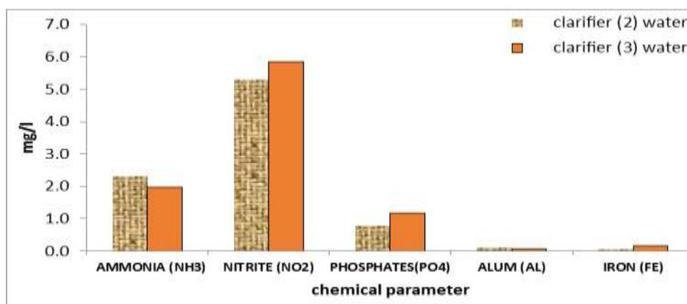
**Figure (2)** Comparison between different clarifiers water produced from El-Asher drinking Water treatment.
