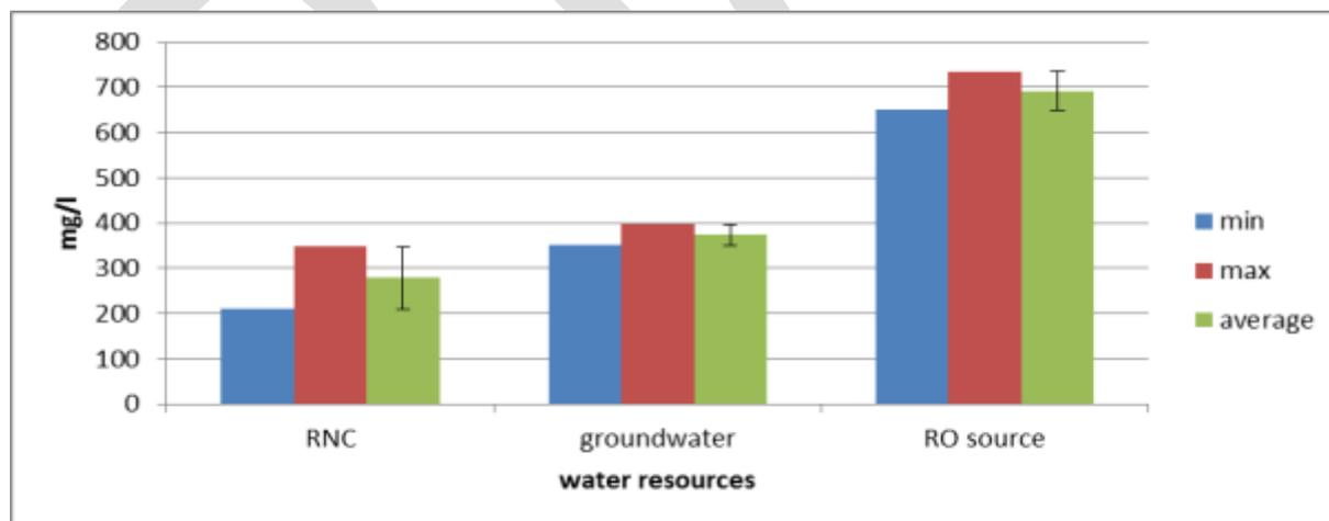
**Figure 1.** Total dissolved solids of different water resources used for drinking water production through studying period of March, 2017 and June, 2018.
